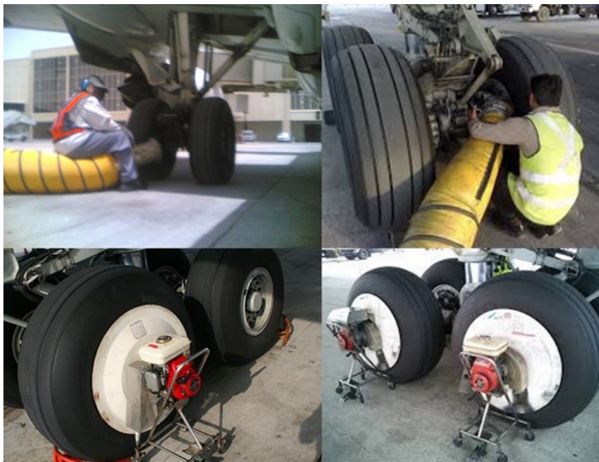
Image 12: Demonstration of an aircraft external cooling system.
