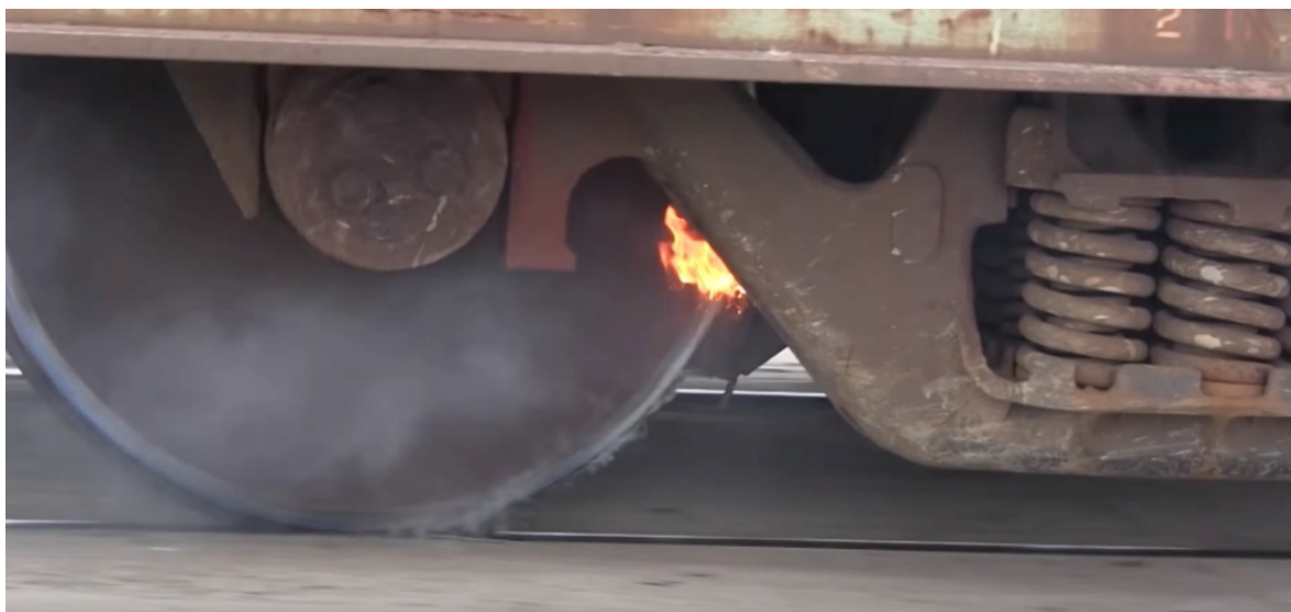
Image 2: Rail transport brake failure.
