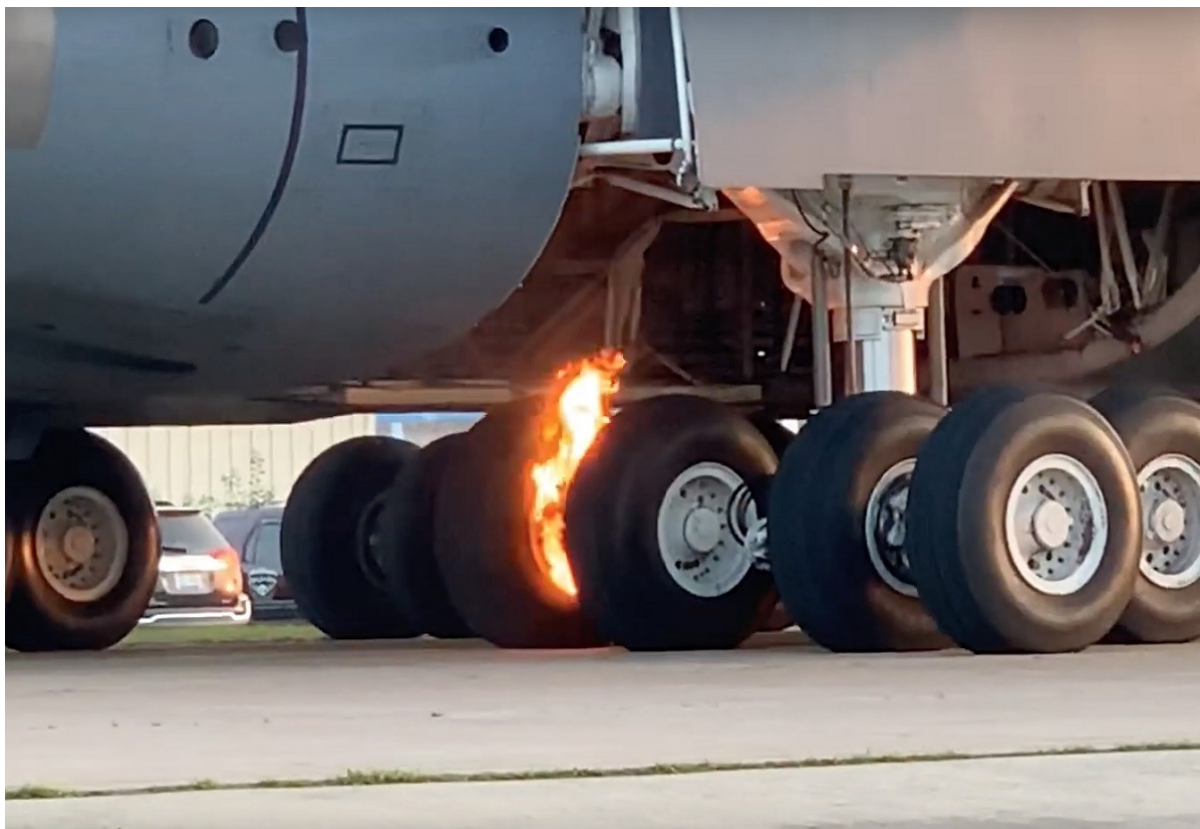
Image 4: Aircraft brake failure during landing.
