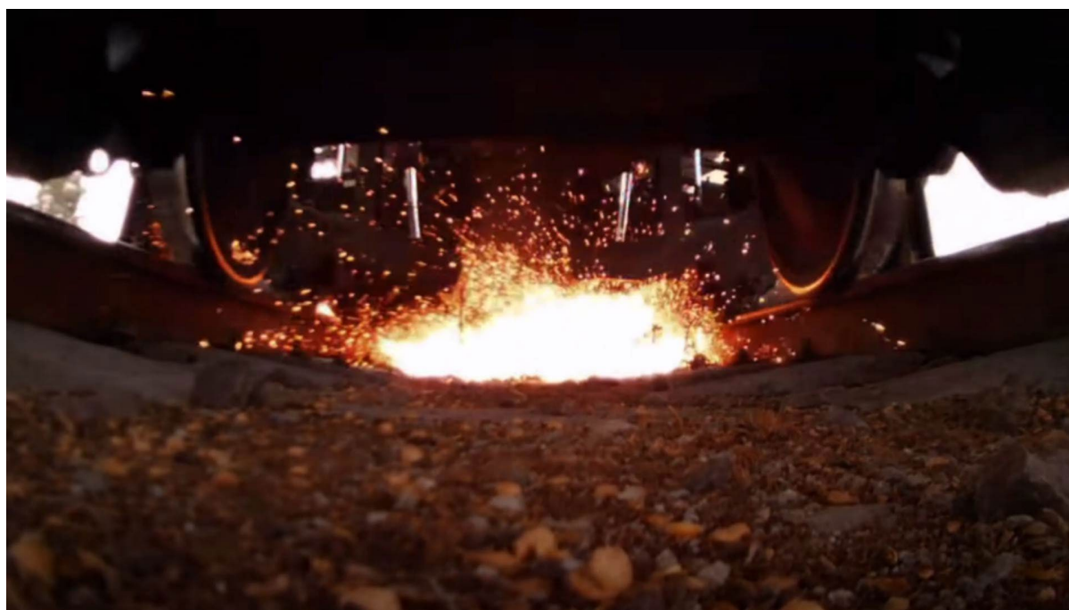
Image 3: Excessive temperatures in train brake assembly.
